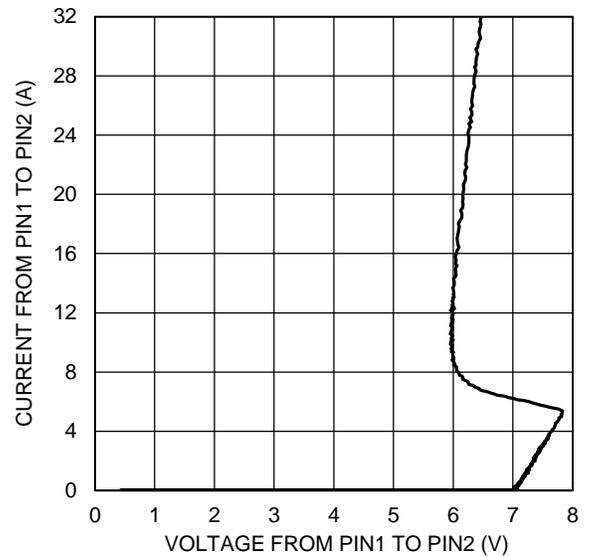
Figure 6 Positive TLP Curve ( $t_p=100ns$ )
