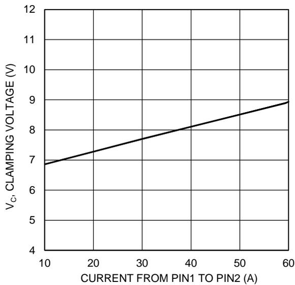
Figure 5 Clamping Voltage Characteristic ( $t_p=8/20\mu s$ )
