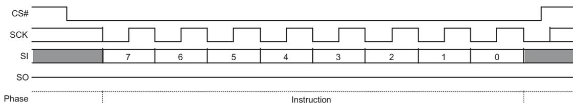
Figure 58. Read Electronic Signature (RES ABh) Command Sequence
