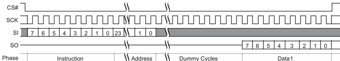
Figure 11. Dual Output Command
