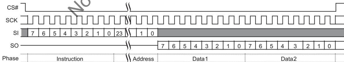
Figure 10. Single Bit Wide I/O Command with Latency
