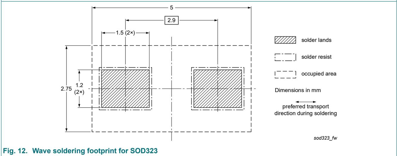
Fig. 12. Wave soldering footprint for SOD323
