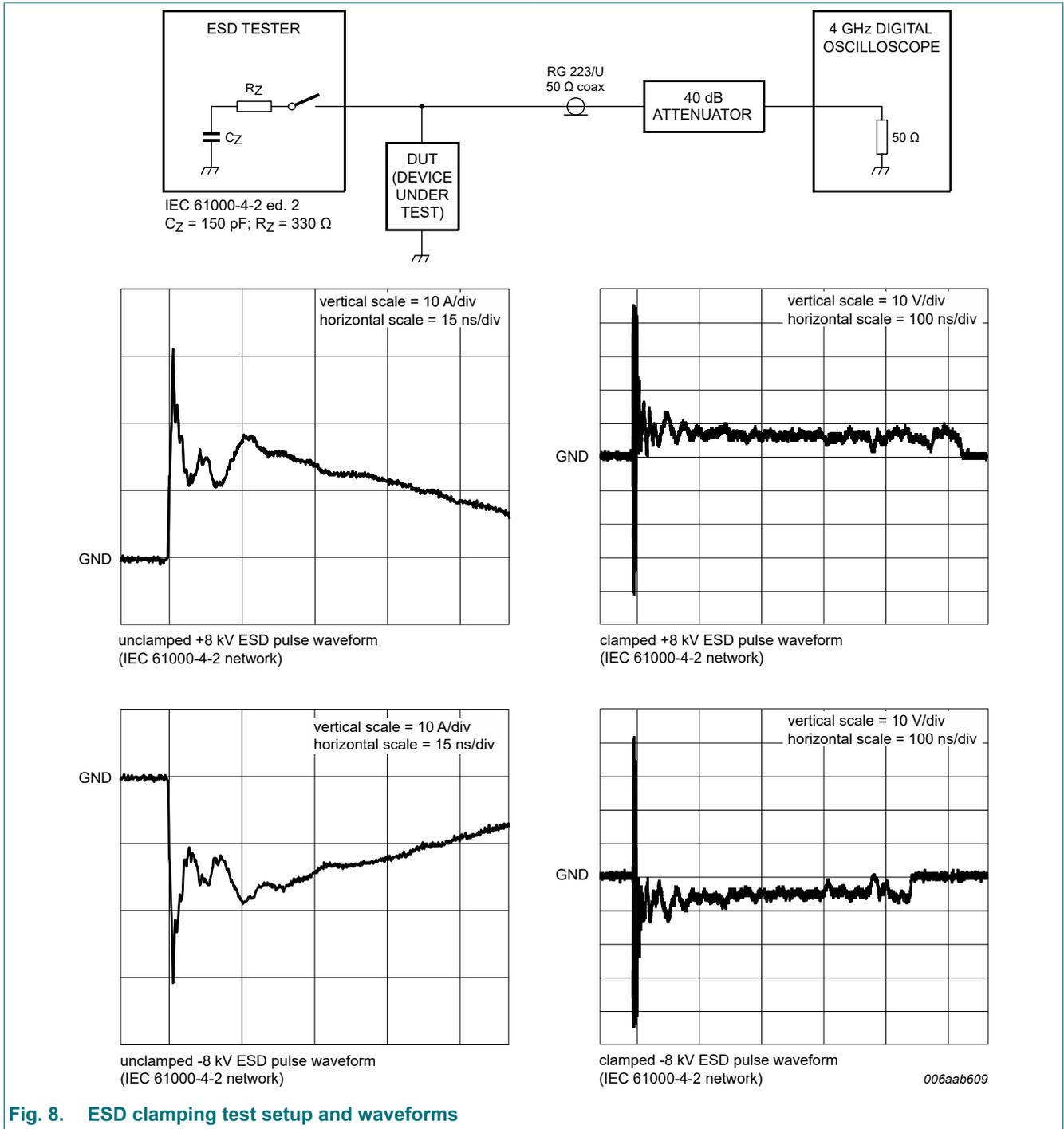
Fig. 8. ESD clamping test setup and waveforms
