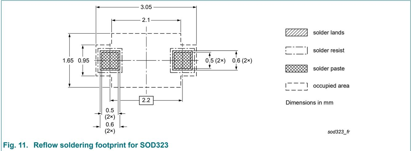
Fig. 11. Reflow soldering footprint for SOD323
