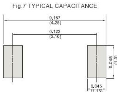
**Mechanical Dimensions SOD-123FL(Inches/Millimeters)**
