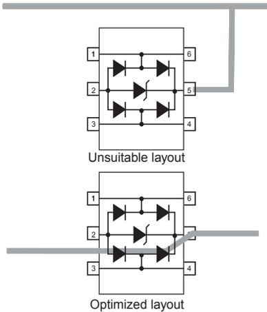
**Figure 7. ESD behavior: measurement conditions**
