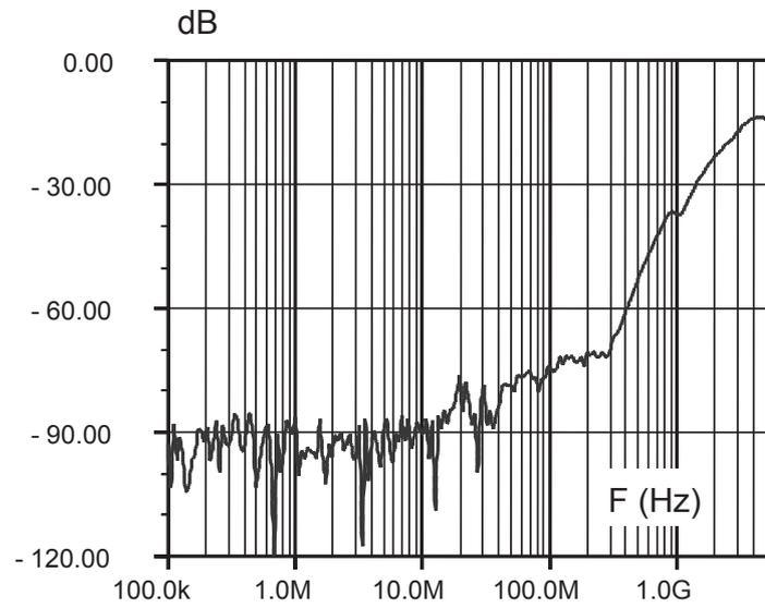
As the USBLC6-2 is designed to protect high speed data lines, it must ensure a good transmission of operating signals. The frequency response (Figure 4. Frequency response) gives attenuation information and shows that the USBLC6-2 is well suitable for data line transmission up to 480 Mbit/s while it works as a filter for undesirable signals like GSM (900 MHz) frequencies, for instance.
