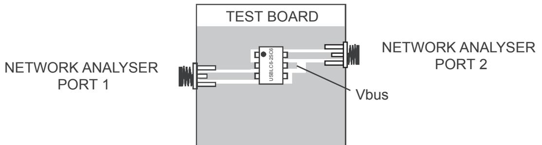
Figure 11. Analog crosstalk measurements shows the measurement circuit for the analog application. In usual frequency range of analog signals (up to 240 MHz) the effect on disturbed line is less than -55 dB (see Figure 12. Analog crosstalk results).
