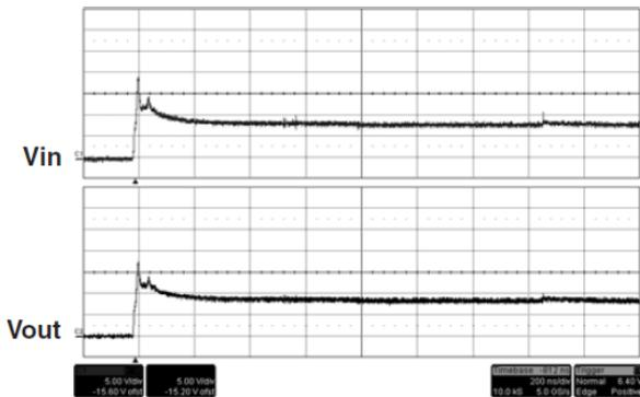
**Figure 9. ESD response to IEC 61000-4-2 (-15 kV air discharge)**
