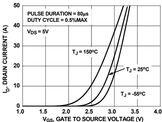
Figure 5. Transfer Characteristics
