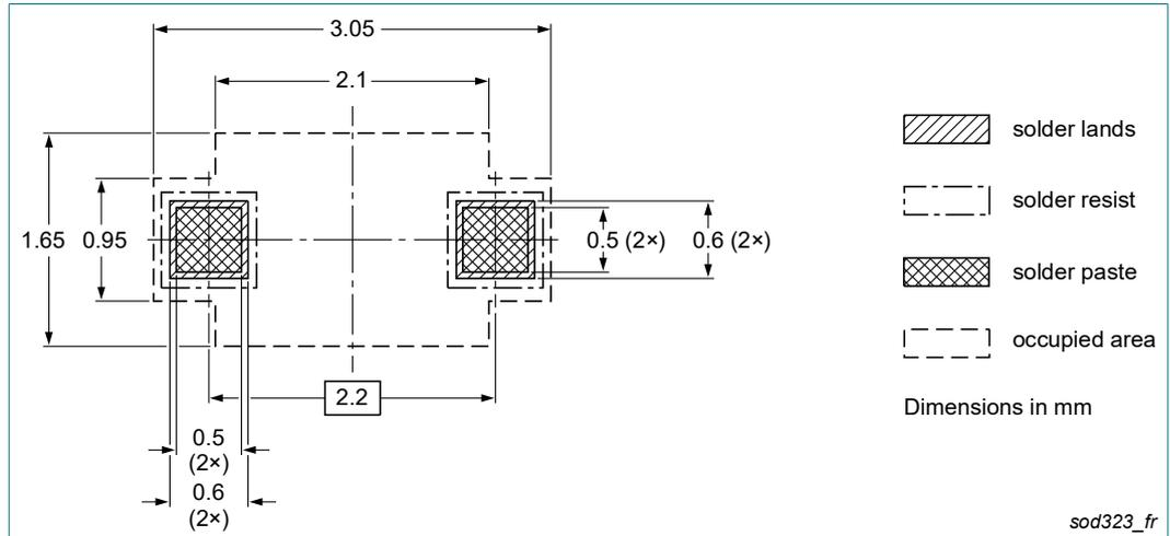
Fig. 12. Reflow soldering footprint for SOD323 (SC-76)
