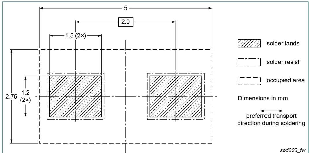
Fig. 13. Wave soldering footprint for SOD323 (SC-76)
