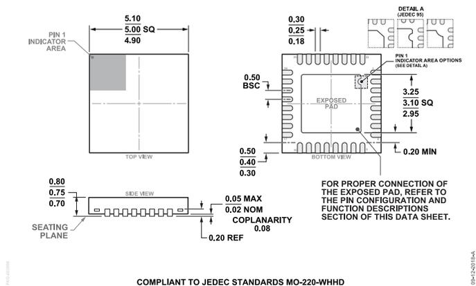
**Figure 91. 32-Lead Lead Frame Chip Scale Package [LFCSP]
