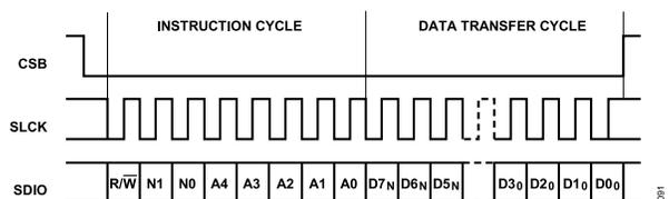
**Figure 71. Serial Register Interface Timing, MSB First Write**
