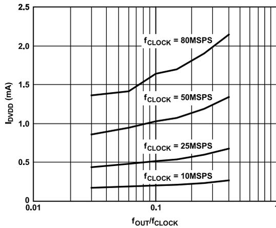
Figure 83.  $I_{DVDD}$  vs.  $f_{OUT}/f_{CLOCK}$  Ratio at  $DVDD = 1.8 V$
