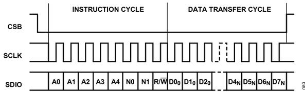
Figure 73. Serial Register Interface Timing, LSB First Write
