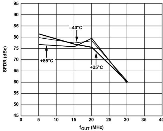
Figure 40. SFDR vs. Temperature at 80 MSPS
