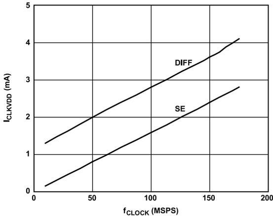
Figure 84.  $I_{CLKVDD}$  vs.  $f_{CLOCK}$  at  $CLKVDD = 3.3 V$
