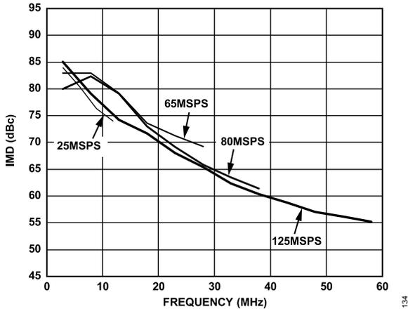
Figure 34. Dual-Tone IMD vs. Lower  $f_{OUT}$  at  $I_{OUTFS} = 1\text{ mA}$  and 0 dBFS
