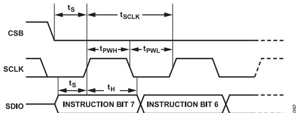
Figure 75. Timing Diagram for SPI Register Write
