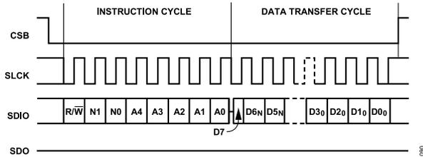
Figure 72. Serial Register Interface Timing, MSB First Read
