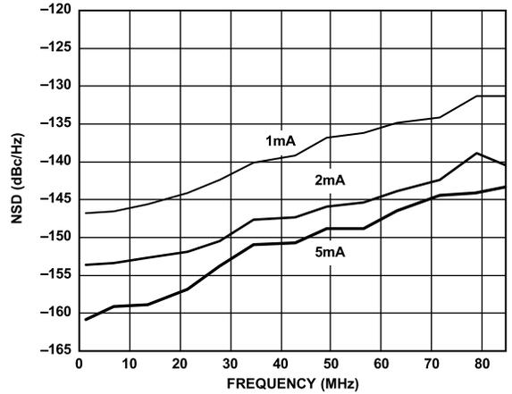
Figure 16. NSD vs.  $f_{OUT}$  and  $I_{OUTFS}$  at 175 MSPS
