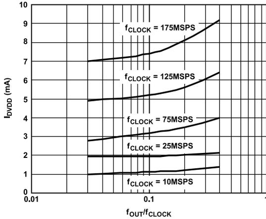
Figure 82.  $I_{DVDD}$  vs.  $f_{OUT}/f_{CLOCK}$  Ratio at  $DVDD = 3.3 V$
