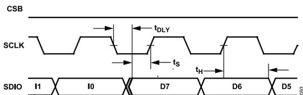
Figure 76. Timing Diagram for SPI Register Read
