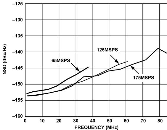
Figure 15. NSD vs.  $f_{OUT}$  and  $f_{CLOCK}$  at 0 dBFS
