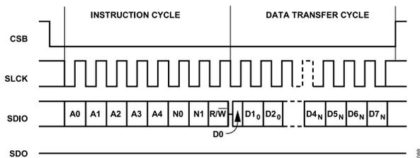
Figure 74. Serial Register Interface Timing, LSB First Read
