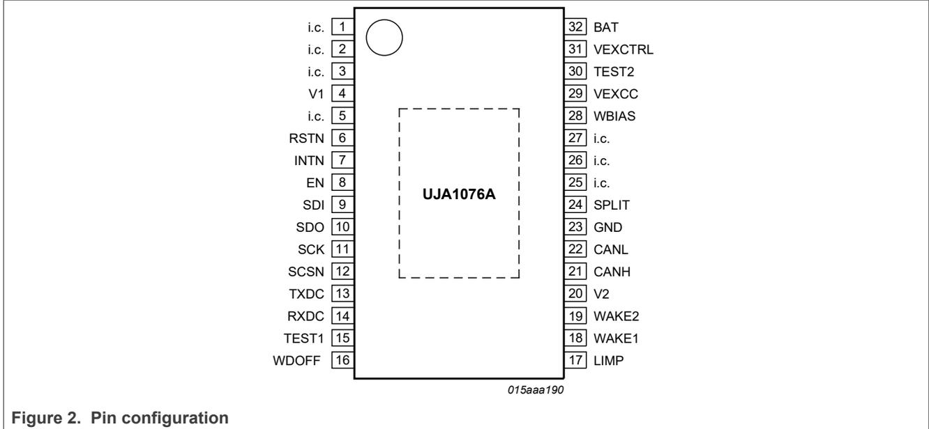
Figure 2. Pin configuration
