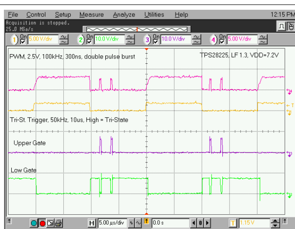
Figure 6-3. 2.5-V Amplitude PWM Pulse
