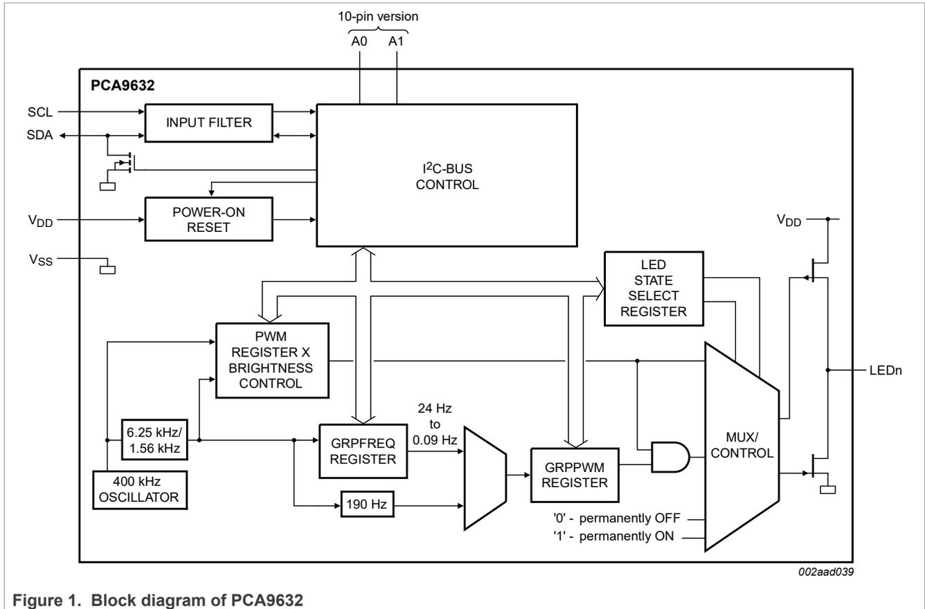
Figure 1. Block diagram of PCA9632
