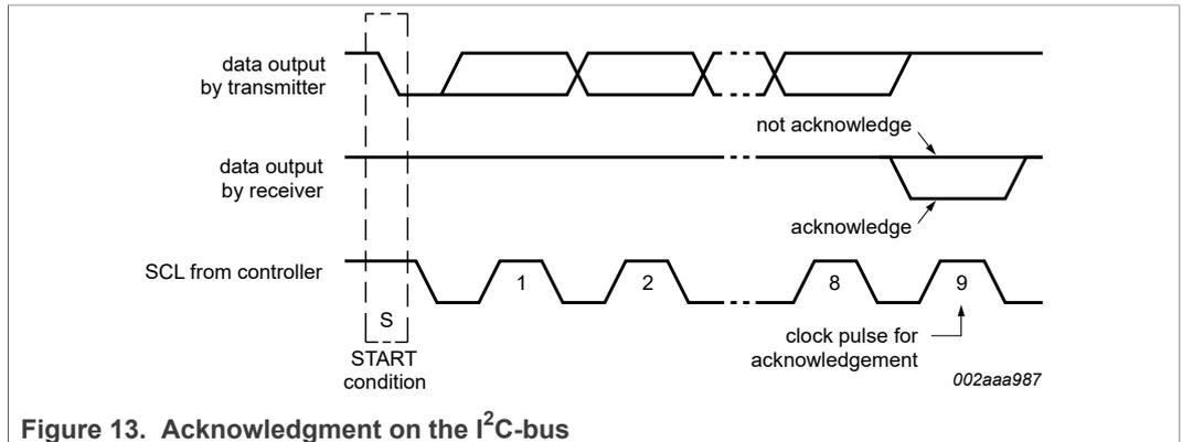
Figure 13. Acknowledgment on the I<sup>2</sup>C-bus
