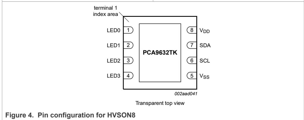
Figure 4. Pin configuration for HVSON8
