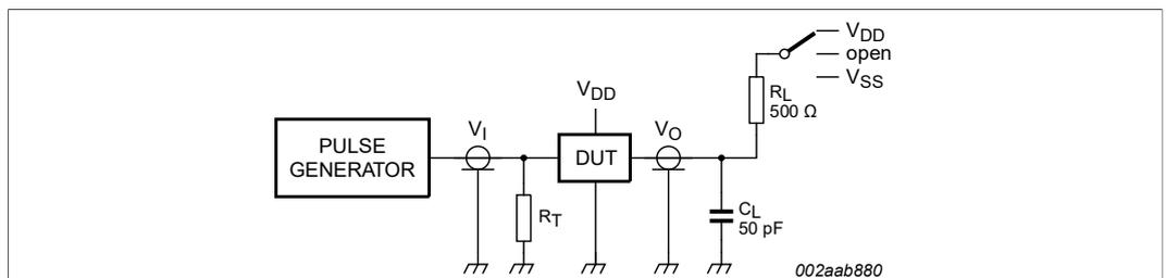
R<sub>L</sub> = Load resistor for LEDn. R<sub>L</sub> for SDA and SCL > 1 kΩ (3 mA or less current).
