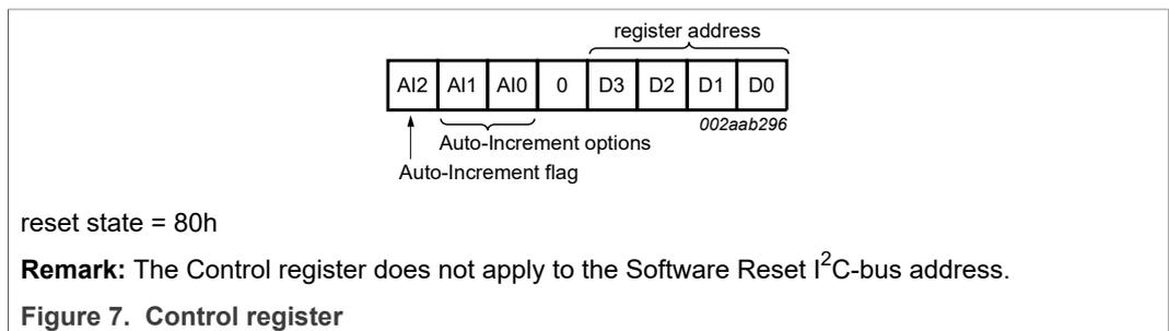
When the Auto-Increment flag is set (AI2 = 1), the four low order bits of the Control register are automatically incremented after a read or write. This allows the user to program the registers sequentially. Four different types of Auto-Increment are possible, depending on AI1 and AI0 values.
