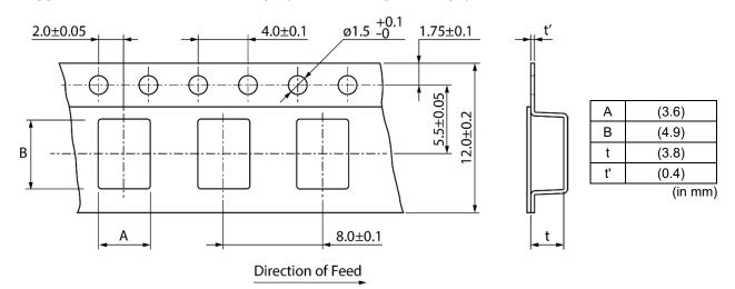
\* The dimensions of the cavity are measured at its bottom.
