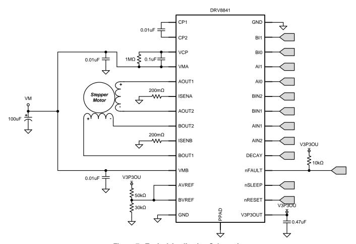
Figure 7. Typical Application Schematic
