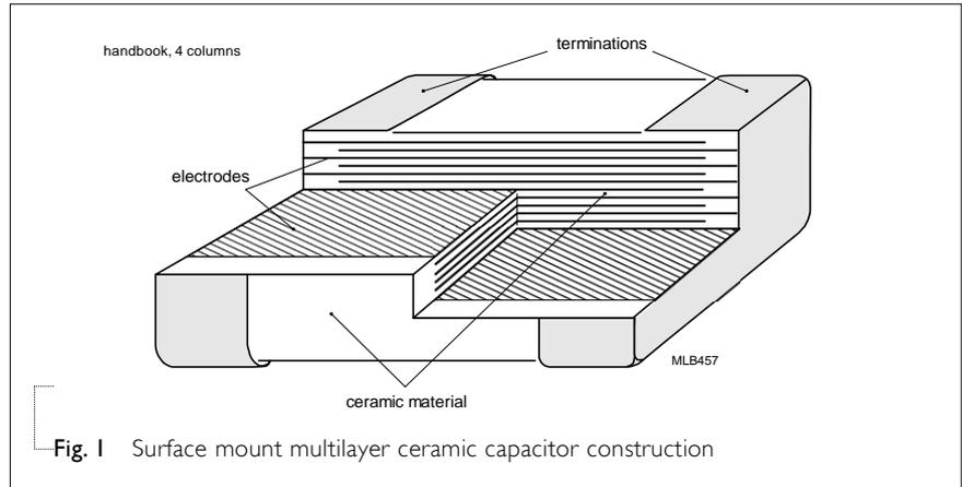
Fig. 1 Surface mount multilayer ceramic capacitor construction
