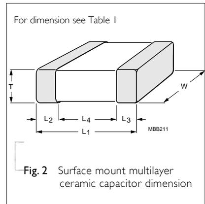
Fig. 2 Surface mount multilayer ceramic capacitor dimension
