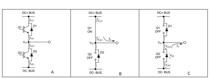
**Figure 21** Figure A shows the Parasitic Elements. Figure B shows the generation of V<sub>s</sub> positive. Figure C shows the generation of V<sub>s</sub> negative
