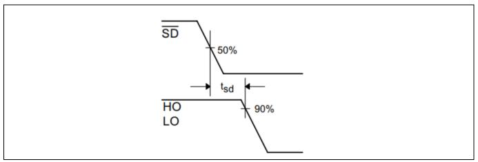
Figure 14 Shutdown waveform definitions
