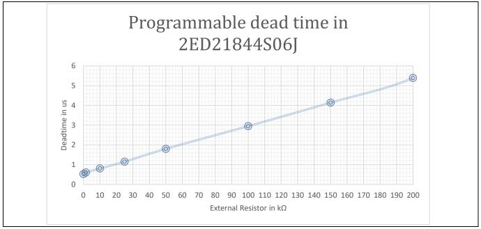
Figure 11 Variation of dead time vs. external resistor
