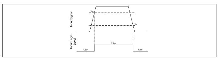
Figure 12 IN input thresholds
