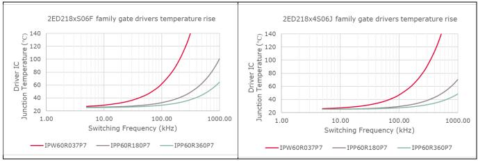
\*Assumptions for above curves:  $T_a = 25 \text{ °C}$ ,  $V_{BUS} = 400 \text{ V}$ ,  $V_{CC} = 12 \text{ V}$ ,  $R_{gon} = 10 \Omega$ ,  $R_{goff} = 5\Omega$
