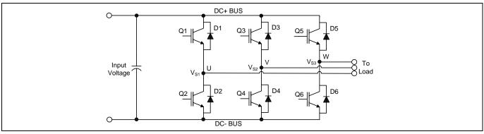
Figure 19 Three phase inverter
