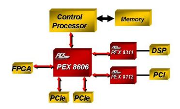
Figure 2. Fan-in/out Usage
