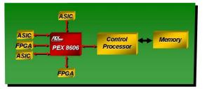
Figure 5. Packet Processing Module
