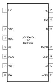
Figure 5-1. DDB Package 16-Pin SOIC (Pins 2, 13 removed) Top View
