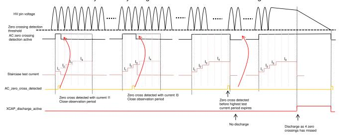
Figure 7-15. Different Staircase Current Waveforms
