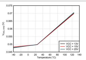
Figure 6-22.  $V_{HOL}$ -  $V_{HS}$  vs Temperature
