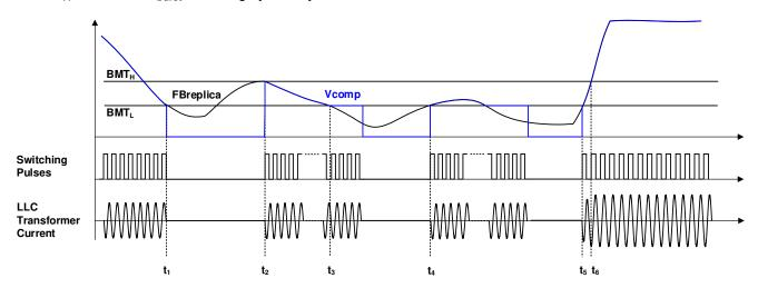
Figure 7-18. Burst Mode Switching Pattern when Soft On and Soft Off is Disabled
