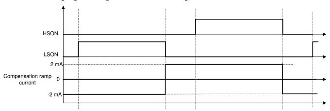
Figure 7-6. VCR Compensation Ramp Current On/Off
