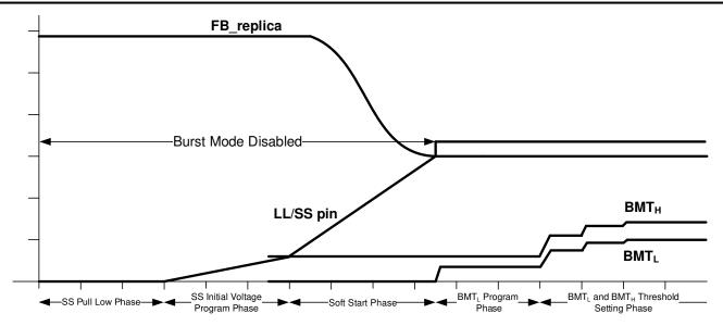
Figure 7-20. Timing Diagram of LL/SS Pin Programming
