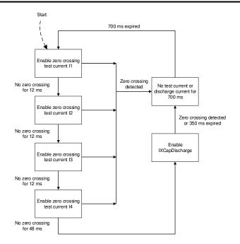
Figure 7-16. AC ZCD and X-Capacitor Discharge Flow Chart
