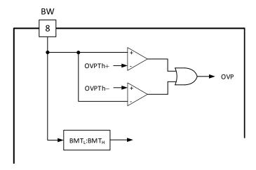
Figure 7-9. Bias Winding Sensing Block Diagram
