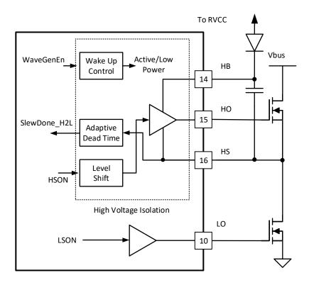
Figure 7-10. Gate Driver Block Diagram
