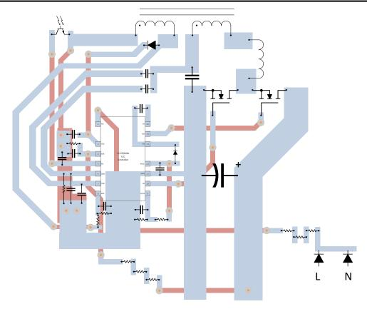
Figure 9-2. Layout Example for Double-Layer PCB
