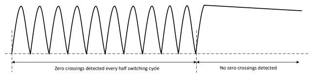
Figure 7-13. AC Disconnect Waveform
