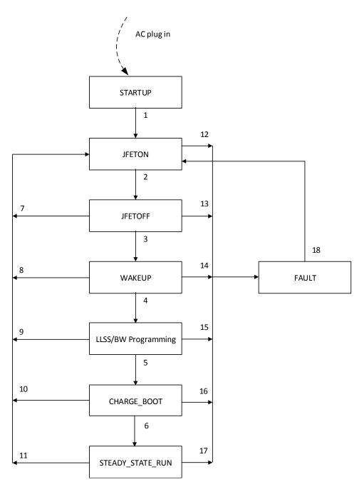
Figure 7-22. System State Machine Transition
