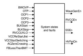
Figure 7-21. Block Diagram of System State Machine
