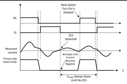
Figure 7-12. Timing Diagram of a ZCS Event
