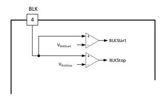
Figure 7-8. BLK Pin Block Diagram
