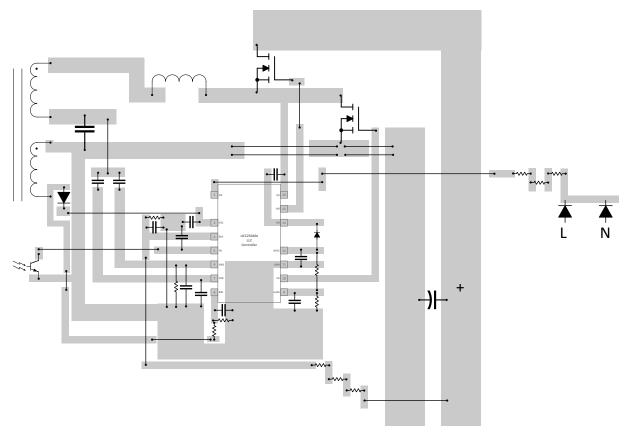
Figure 9-1. Layout Example for Single-Layer PCB
