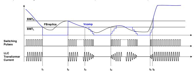
Figure 7-17. Burst Mode Switching Pattern
