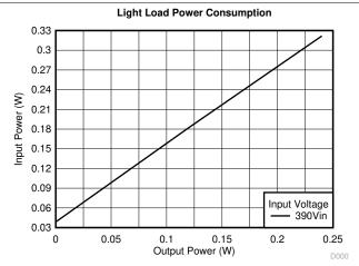
Figure 8-2. Light Load Power Consumption
