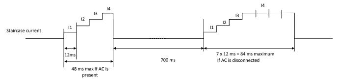
Figure 7-14. Staircase Test Current for X-Capacitor Discharge
