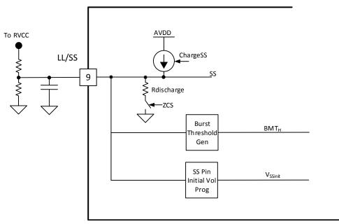
Figure 7-19. LL/SS Block Diagram
