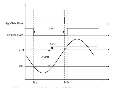
Figure 7-2. HHC Gate On/Off Control Principle
