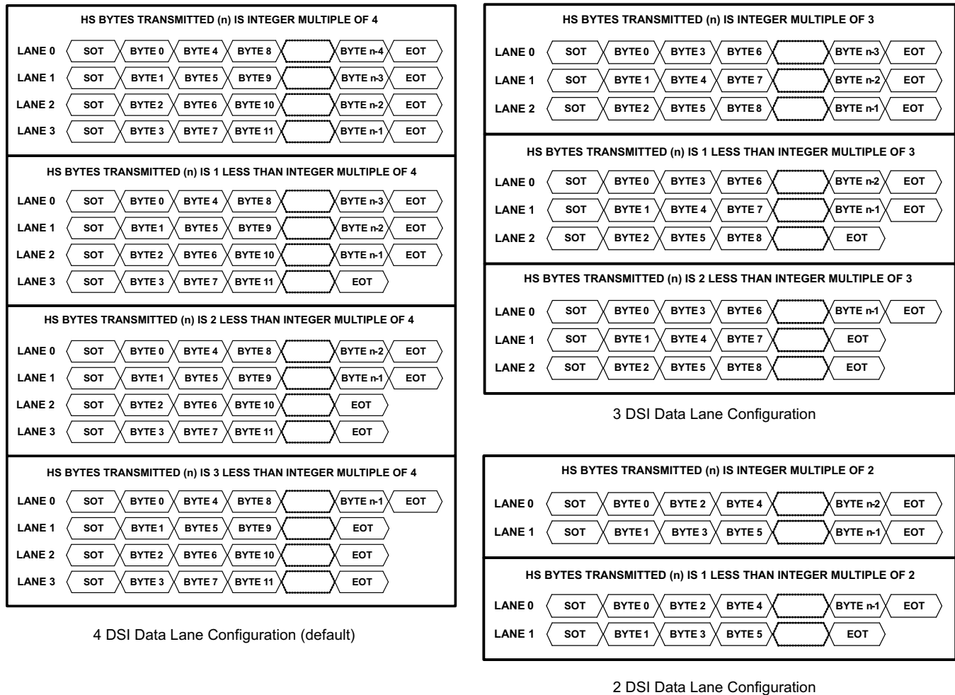
Figure 13. SN65DSI85-Q1 DSI Lane Merging Illustration
