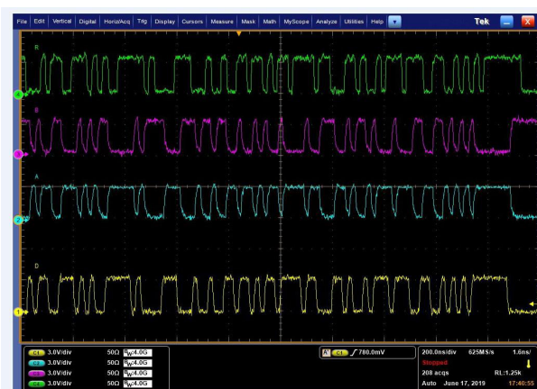
THVD2450 V_{CC} = 3.3\text{ V} R_L = 50\ \Omega Random (PRBS7) data at 50 Mbps
